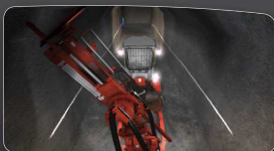
Inclined Fan Drilling
