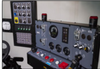
Jacks and tramming controls
