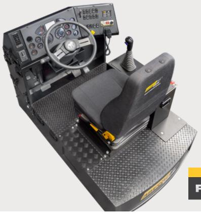
OEM Steering wheel and switches simulating a cabin with the steering wheel on the left side
