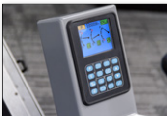
Vehicle Monitoring Screen and Keypad
