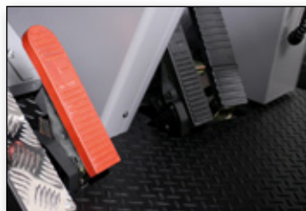
Accelerator, Service Brake and Secondary Brake layout matches real machine
