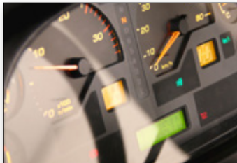
Genuine HD785-7 dash including Komatsu steering wheel, engine tachometer, speedometer and LCD unit
