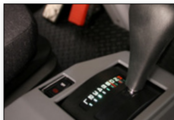
Gear Shift lever, lock and Park Brake switch
