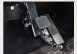
Komatsu throttle and blended retarder/hydraulic brake pedal.
