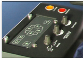
IDU keypad and functional indicators
