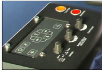
IDU keypad and functional indicators
