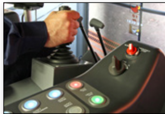
Dual axis boom/bucket control joysticks and functional switch panel
