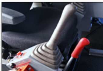
Dual axis control joysticks and functional lock lever
