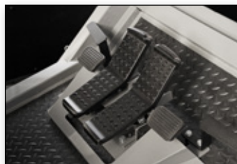
Bucket and track pedals match real machine cab
