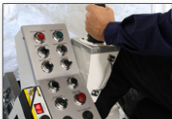
Dual axis bucket control joysticks and functional switch panel
