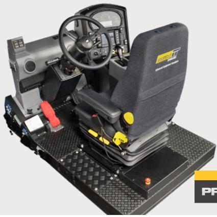
Genuine gauges and speedometer with simulated Caterpillar® Advisor system LCD display
