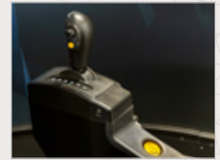
Genuine shift lever and park brake safety switch.
