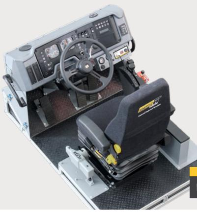
Genuine gauges, speedometer and Caterpillar® Electronic Monitoring System (CEMS)
