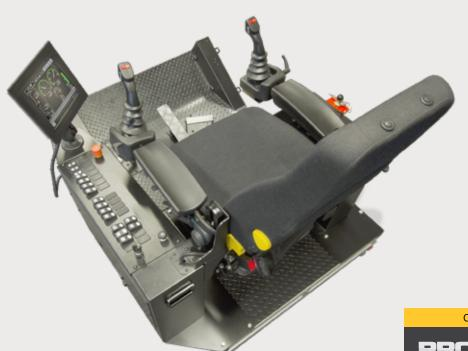
Emulated Board Control System (BCS) touch screen panel which displays essential vehicle status information and faults.
