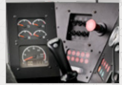
Caterpillar® Electronic Monitoring System (CEMS) with message center, gauges & switch panel
