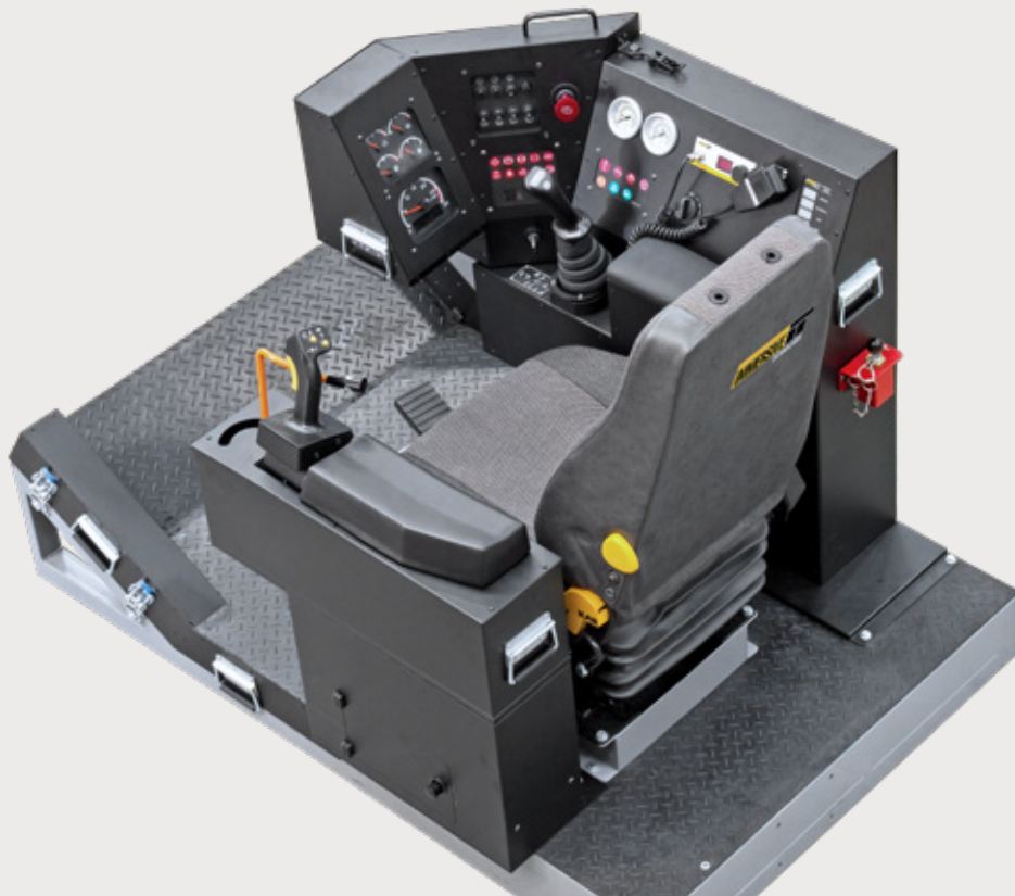
Caterpillar® Electronic Monitoring System (CEMS) with message center, gauges & switch panel
