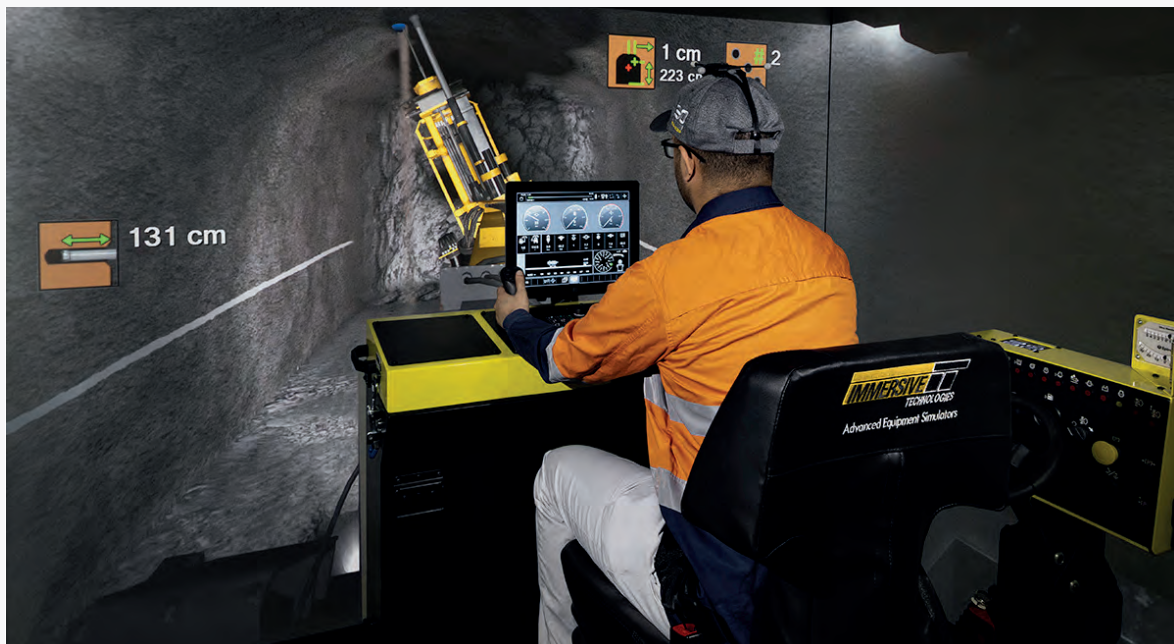
IM360+ Advanced Equipment Simulator equipped with a Epiroc Production Drill Conversion Kit®
